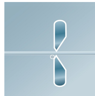
Figure 3-72 Incorrect Blade Placement
