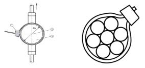
The loop tensile strength tests conducted on Type 2 and Type 21 cable ties include a maximum slippage restriction. These cable ties must retain 100% of their declared loop tensile strength after being subjected to specified environmental conditions. Type 1 and Type 11 cable ties must attain 100% of the declared loop tensile strength in the as-received condition, and retain at least 50% of the declared loop tensile strength after being subjected to specified environmental conditions.
