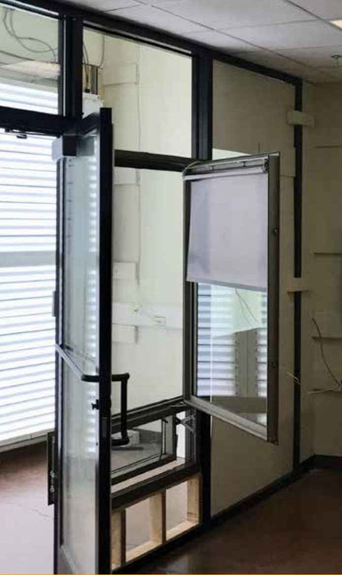
The CLTC Daylight Harvesting Optimization laboratory showing the interior façade and the installation of the electrochromic glazings and the openable window with the roll-down shade, the venting skylight with the solar shade, and the HVAC system. The vertical façade and the skylight are illuminated with controllable electric lighting that is used to simulate daylight changes, such as sunrises, sunsets, partly cloudy skies and uneven distribution of daylight on the façade that can be caused by outdoor obstructions. Photo courtesy of the CLTC
