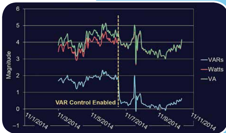
An example of volt/VAR optimization for a specific feeder. Photo courtesy of SEL
