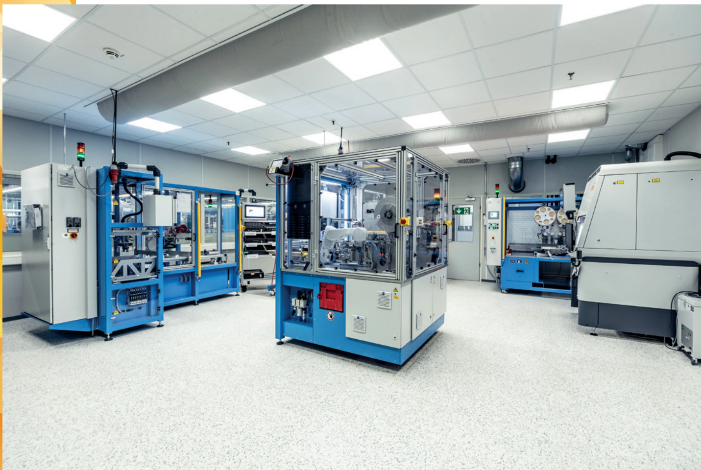
Part of the production line for the ABB-tacteo KNX control element for smart buildings. Established production line concepts struggle with small lots sizes. However, Industry 4.0 concepts such as the digital twin and M2M protocols allow complete flexibility right down to a lot size of one. All photo courtesy of ABB.
