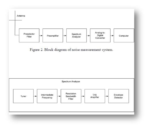
Figure 11. Diagram describing the noise factor equipment setup.
