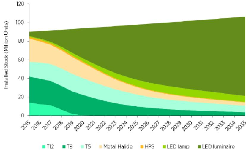
Figure 3, Area and Roadway LED adoption forecast showing MH usage reduction
