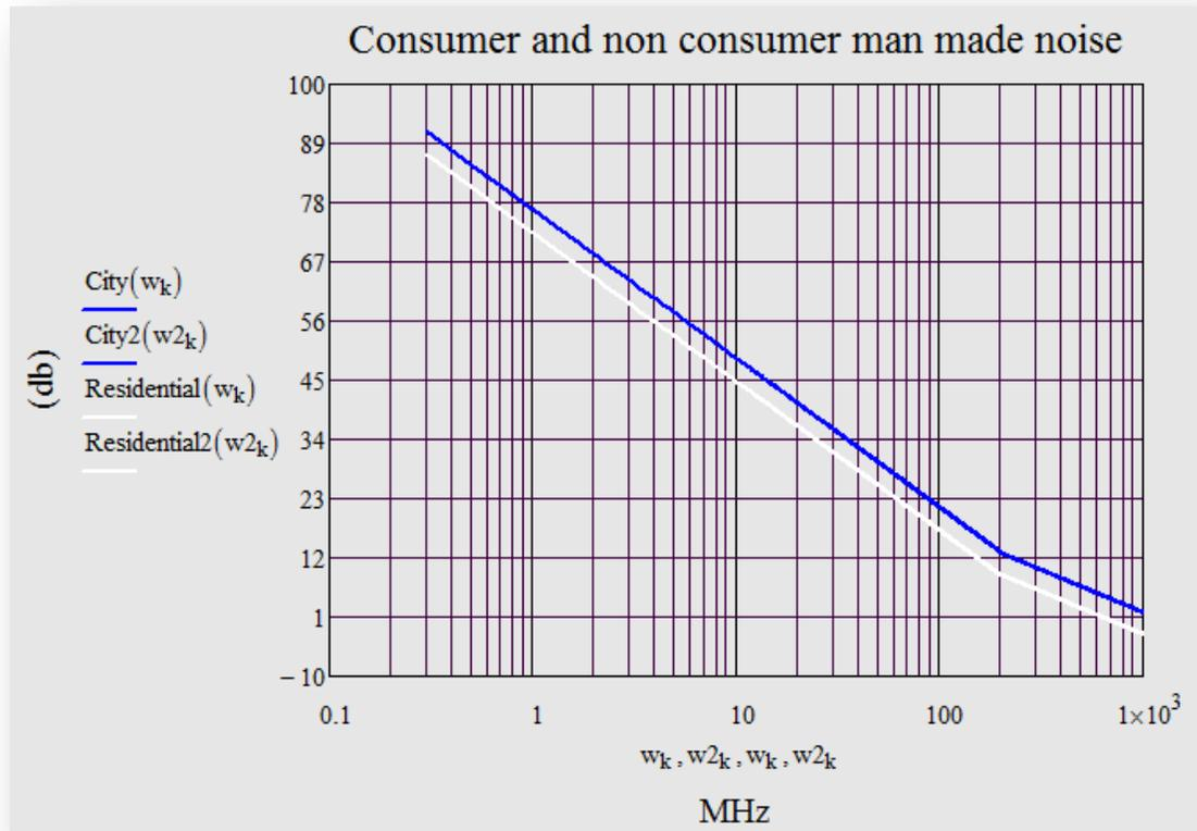
Figure 4. Illustration detailing consumer and non-consumer man-made noise.
