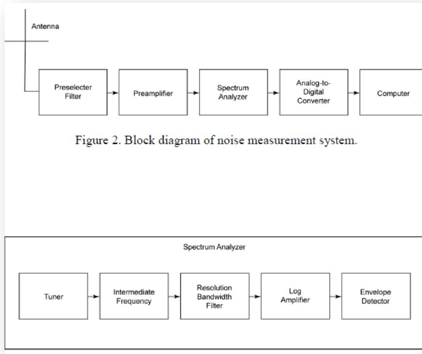
Figure 2. Block diagram of noise measurement system.
