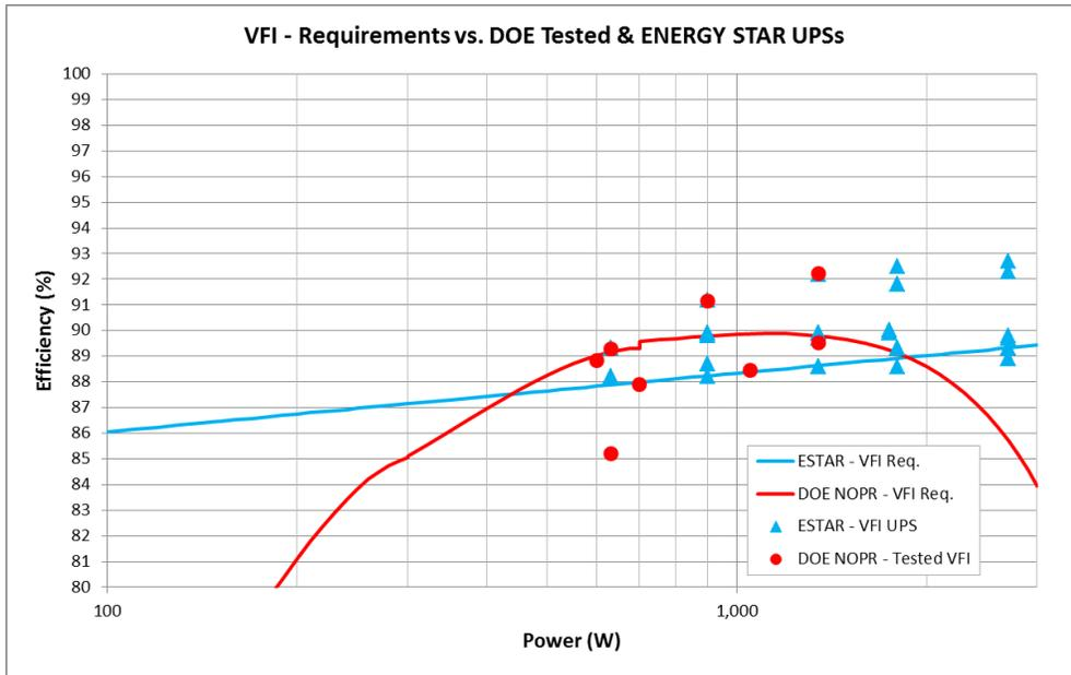
Figure 6: ENERGY STAR and DOE Tested VFI UPS Efficiencies vs. DOE Proposed Curve
