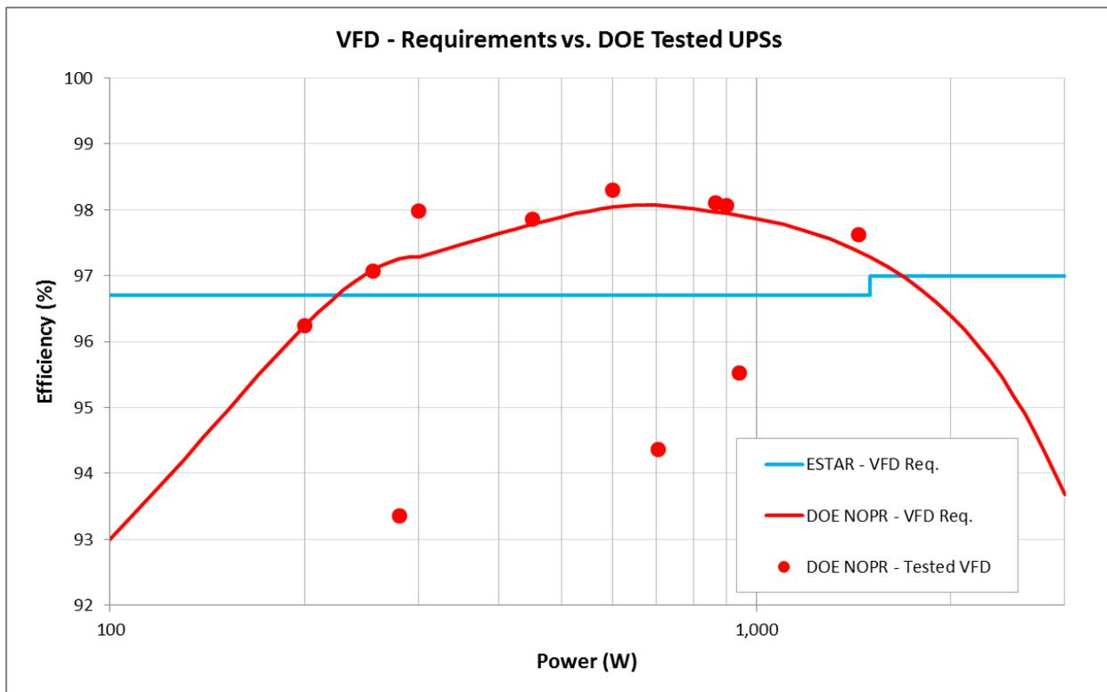
Figure 1: DOE Tested VFD Efficiencies and the DOE Proposed Curve
