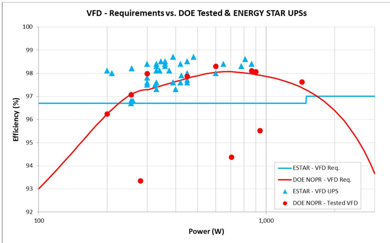
Figure 2: ENERGY STAR VFD Product Efficiencies vs. DOE Proposed Curve
