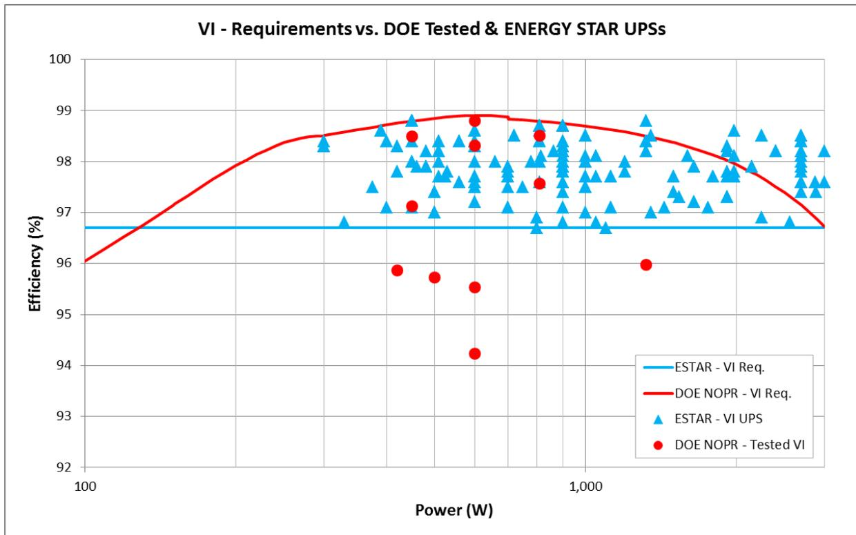
Figure 4: ENERGY STAR and DOE Tested VI UPS Efficiencies vs. the DOE Proposed Curve
