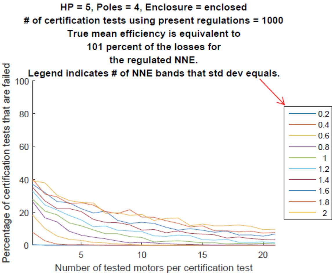
**Figure 8: Percentage of 1000 simulated certification tests per sampling size and per value of standard deviation that were failed for a 5 HP, 4 pole, enclosed electric motor design with a true mean efficiency equivalent to losses 3% higher than those for the 89.5% efficiency mandated by the energy conservation standards when the certification test criteria presently**
