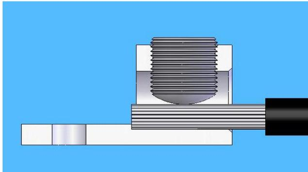
7. Insert the conductor(s) and tighten all set screws per the manufacturer's recommendations.
