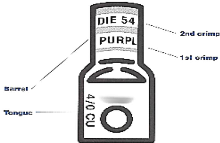
4. Locate tool with correct die in proper position on connector and activate tool
