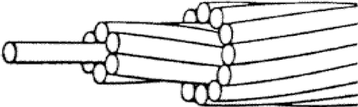
➤ Stranded conductors can be unilay or reverse-lay stranded (or other geometric configuration), and can be concentric, compressed, rope-lay, bunch or compact stranded.
