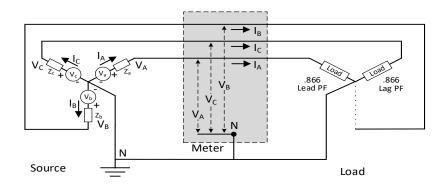
Figure 7 4-Wire Y, One Lead and One Lag PF Load
