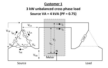
Figure 13 3-Wire Delta, Single Cross Phase Load
