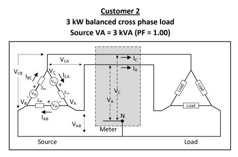
Figure 14 3-Wire Delta, Balanced Cross Phase Load
