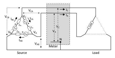
Figure 8 3-Wire Delta, Single Phase to Phase Load
