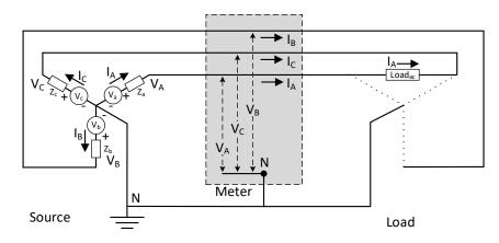
Figure 6 4-Wire Y, Single Cross Phase Load
