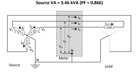
Figure 11 4-Wire Wye, Single Cross Phase Load
