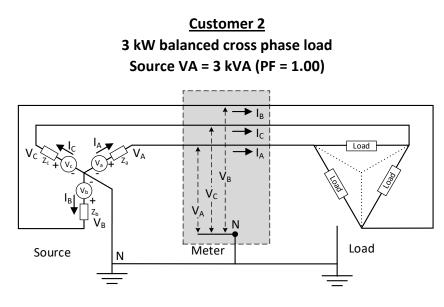
Figure 12 4-Wire Wye, Balanced Cross Phase Load
