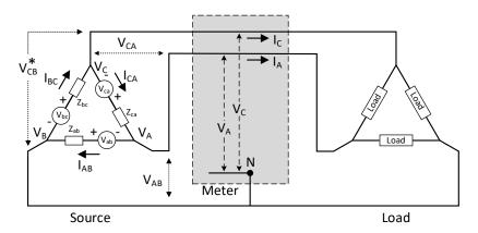
\*This voltage is labeled as  $V_{CB}$  (rather than  $V_{BC}$ ) because this is as viewed by the electric meter.
