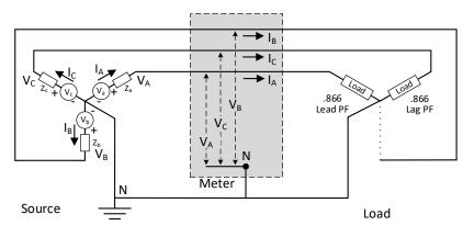
Figure 10 Unbalanced per Phase PF
