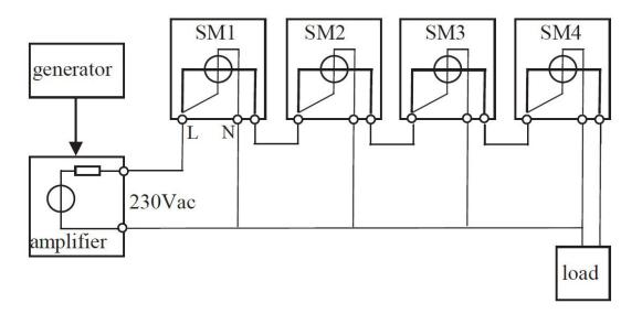
\* With the style meter that was tested, the current (A) is also flowing through the meter's voltage signal input, thus negatively influencing the outcome of the test
